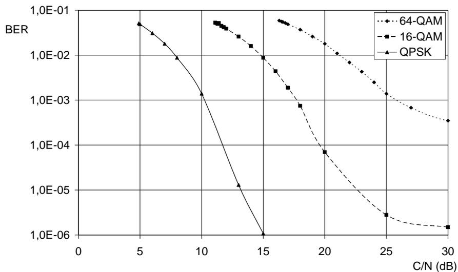
**Figure 4:** Measured dependence of BER before Viterbi decoding on Carrier-to-Noise ratio.
