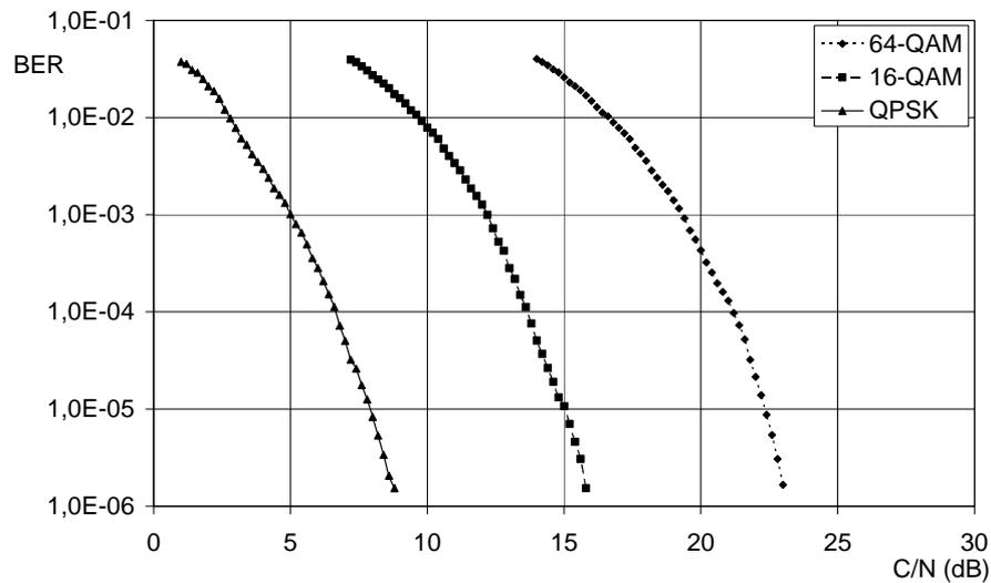
**Figure 3:** Simulated dependence of BER before Viterbi decoding on Carrier-to-Noise ratio.
