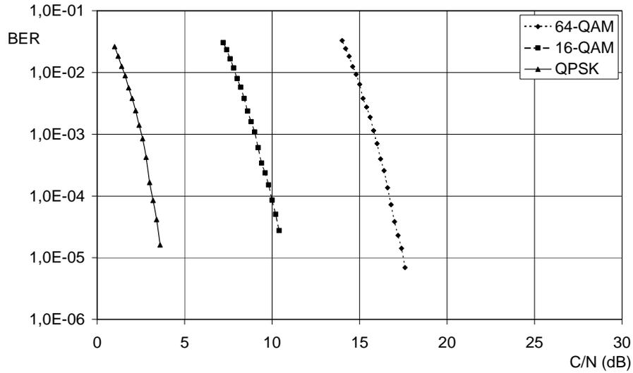
**Figure 5:** Simulated dependence of BER after Viterbi decoding on Carrier-to-Noise ratio.
