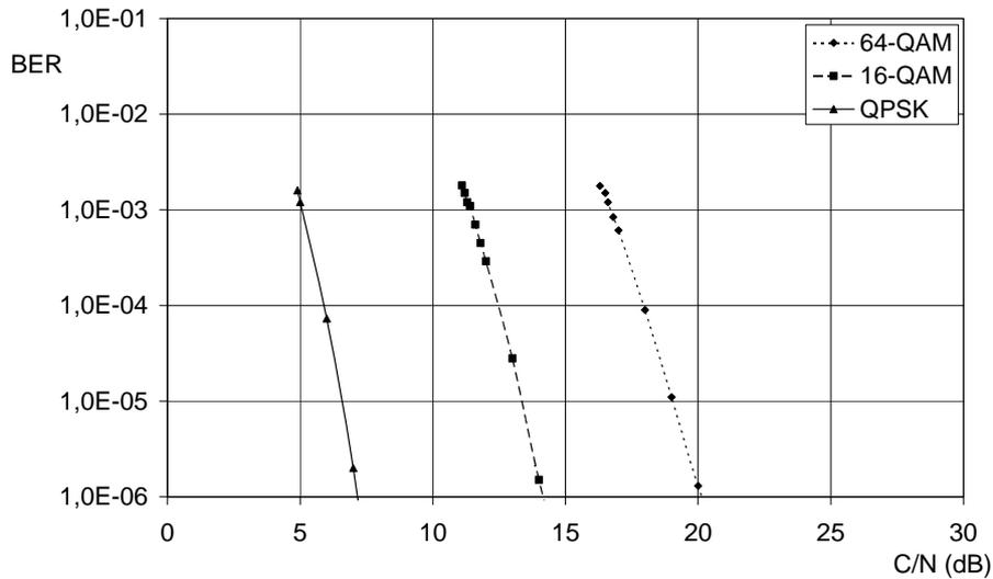
**Figure 6:** Measured dependence of BER after Viterbi decoding on Carrier-to-Noise ratio.
